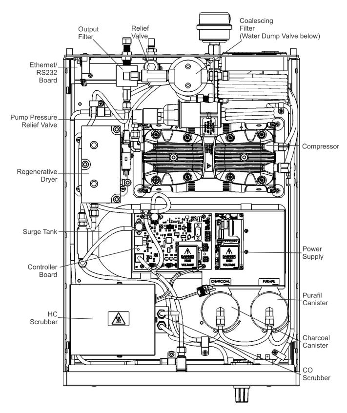
Figure 3-4. N701H Internal Layout
