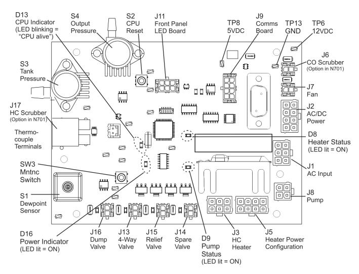
Figure 4-2. Control Board Layout
