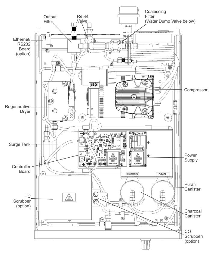
Figure 3-3. N701 Internal Layout (with options)
