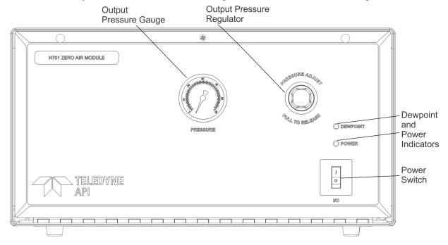
Figure 3-1. Front Panel (N701 label shown)
